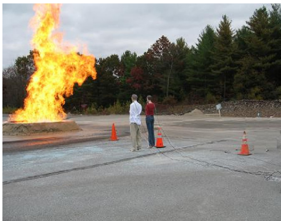
Fig. 4. Mannequins facing the 3 m × 3 m LNG pool fire in an earthen dike.
