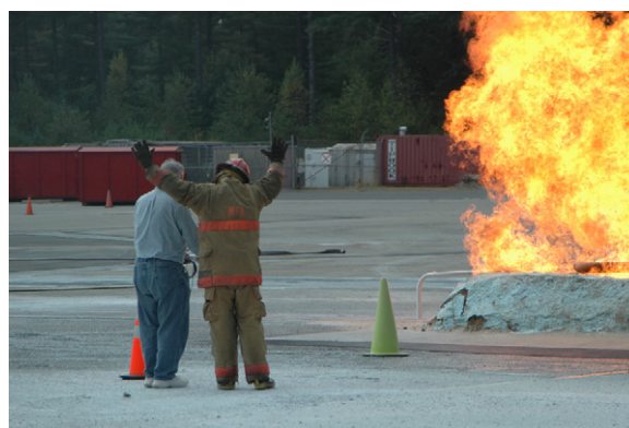
Fig. 7. Author located at about 10 m from fire center holding the hand-held radiometer; fireman's raised arms indicate the reading by the radiometer to be 5 \text{ kW/m}^2 .
