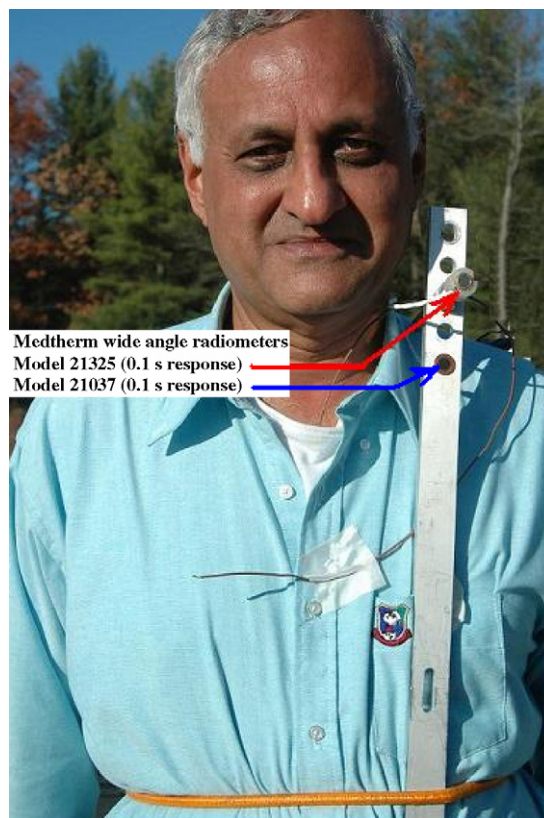
Fig. 6. Illustration of the placement of recording radiometers on the author.
