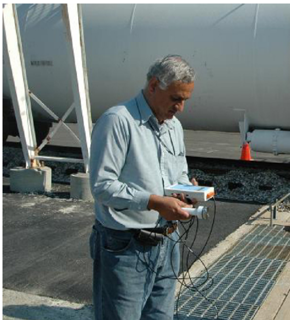
Fig. 5. Hand-held radiometer and illustration of its use in the tests.
